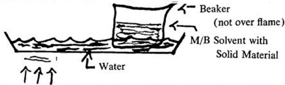
Figure 8. Heating DMT solution in water bath.
